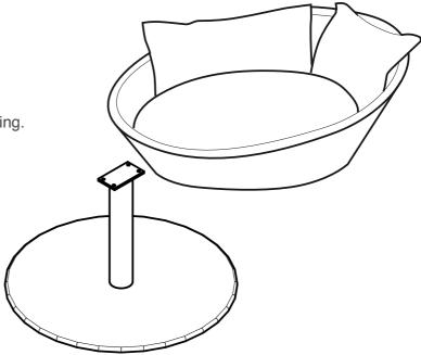
Please unscrew the nuts of the screws at the bottom plate of the top part and set the top part in such a way on the mouting plate of the base, that the screws fit into the drillings of the mounting plate.
